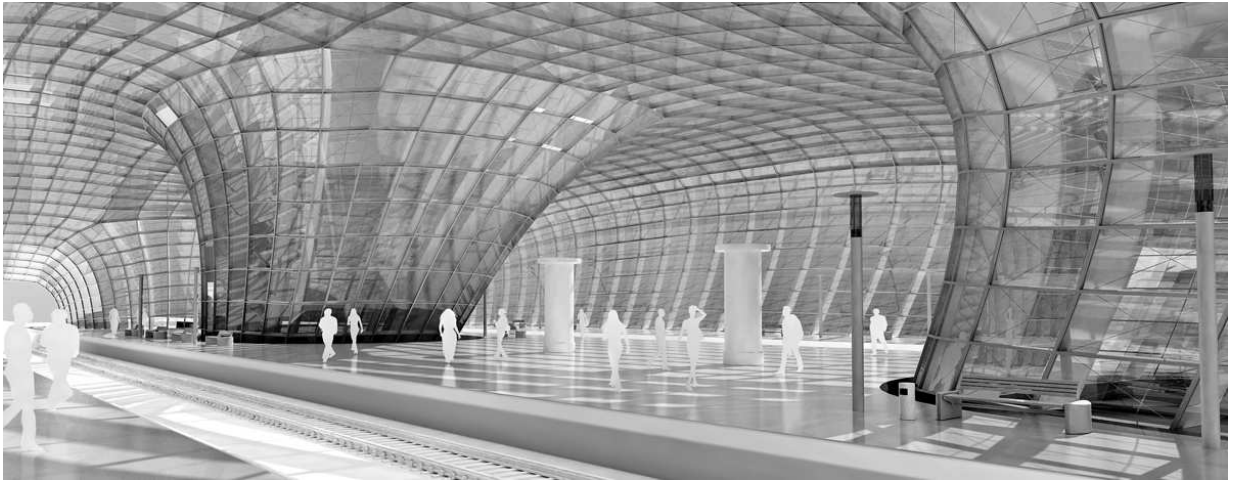
Figure 1: Architectural design based on a conical mesh; part of this image appeared on the front cover of the SIGGRAPH 06 Proceedings issue of ACM Transactions on Graphics .
